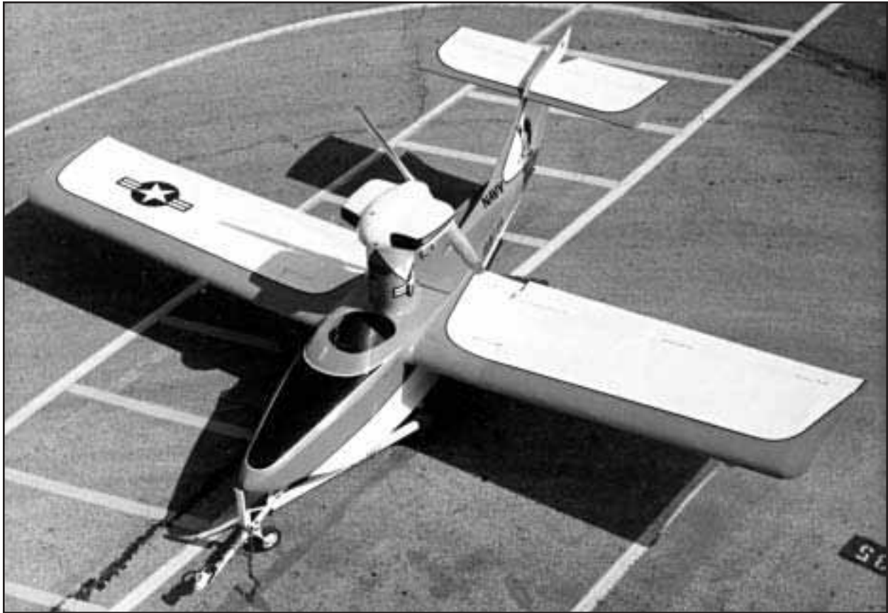
The X-28A was equipped with a simple constant-chord wing. The entire trailing edge, except for a small area near the root, was occupied by flaps and ailerons. The small size of the cockpit is noteworthy. (Howard Levy via the Jay Miller Collection)
