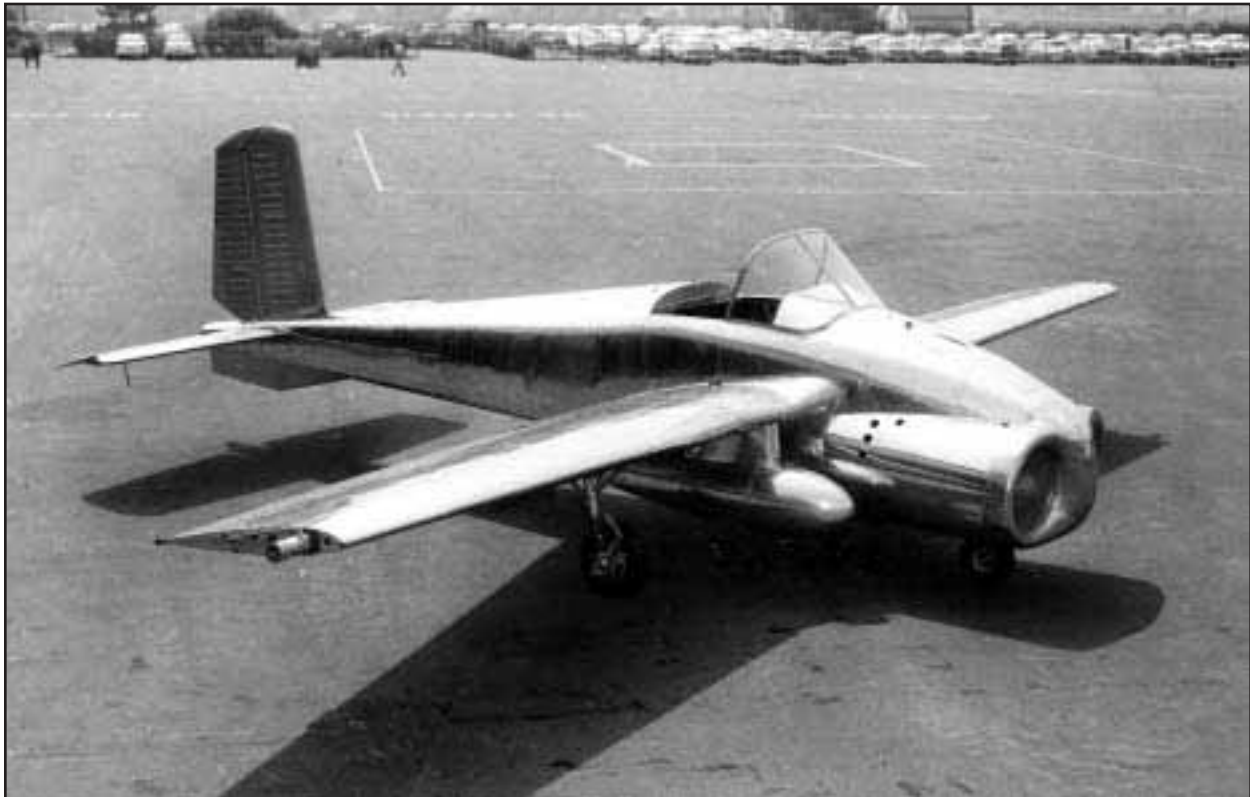
The X-14 was used to verify that the concept of using vectored thrust in a VTOL aircraft was practical. Sir Stanley Hooker would later use this data when designing the Hawker P.1127 (Harrier prototype). (Bell Aerospace via the Jay Miller Collection)
